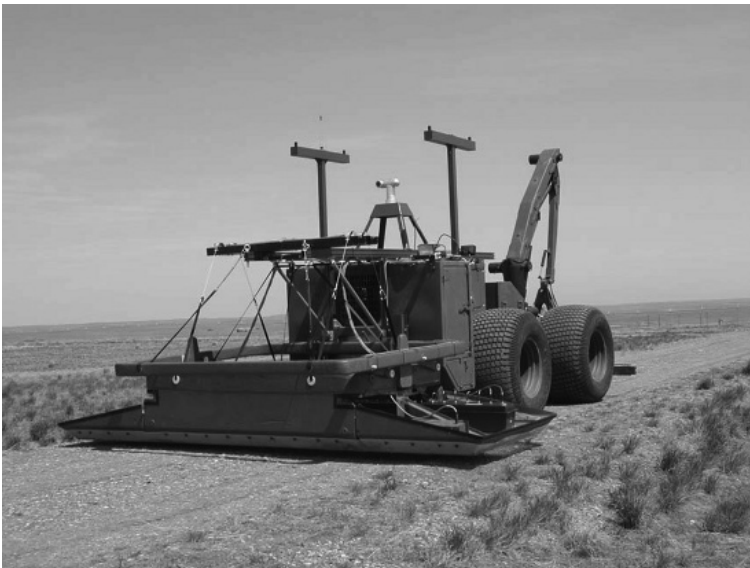
Figure 4.30 Photograph of downward-look, 32-channel array system used on MINDER system ( Courtesy: ERA technology ).
