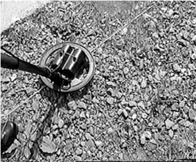
Figure 14.8 Photo of the MINETECT system with a video impulse (Courtesy: ERA Technology (Courtesy Dr. D. Daniels)). Two shielded dipole antennas are seen within the coil of a metal detector.
