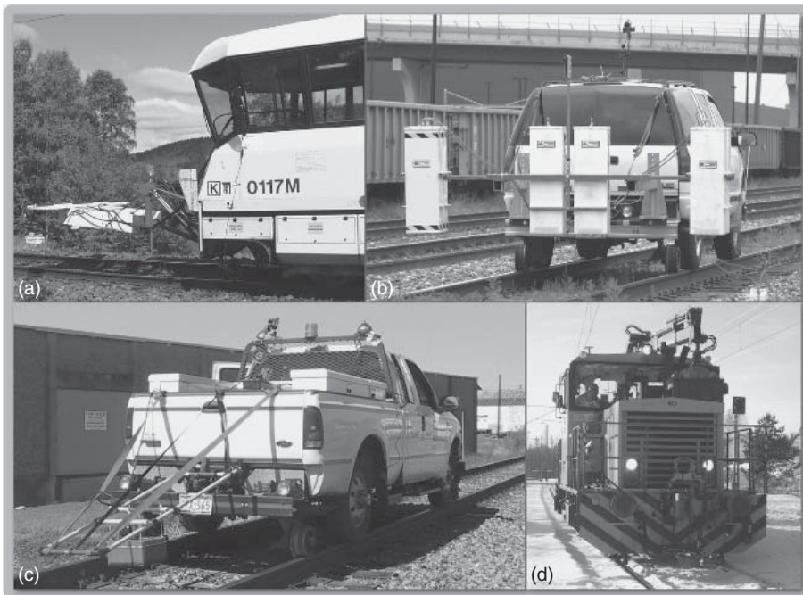
Figure 13.16 Different GPR antennas used in railway surveys. Photo (a) presents a Swedish Mala ground-coupled antenna, photo (b) presents a multichannel GSSI air-coupled system (from Olhoeft et al., 2004), photo (c) presents a GSSI 400-MHz ground-coupled antenna and photo (d) presents Radar Team Sweden 350 MHz 1.2 GHz Sub-Echo HBD antennas.
