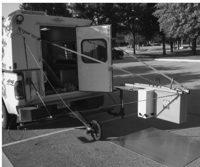
Figure 13.13 Dual polarization configuration of horn antennas for high-speed, high-resolution bridge deck surveys (photo Francisco Romero).
